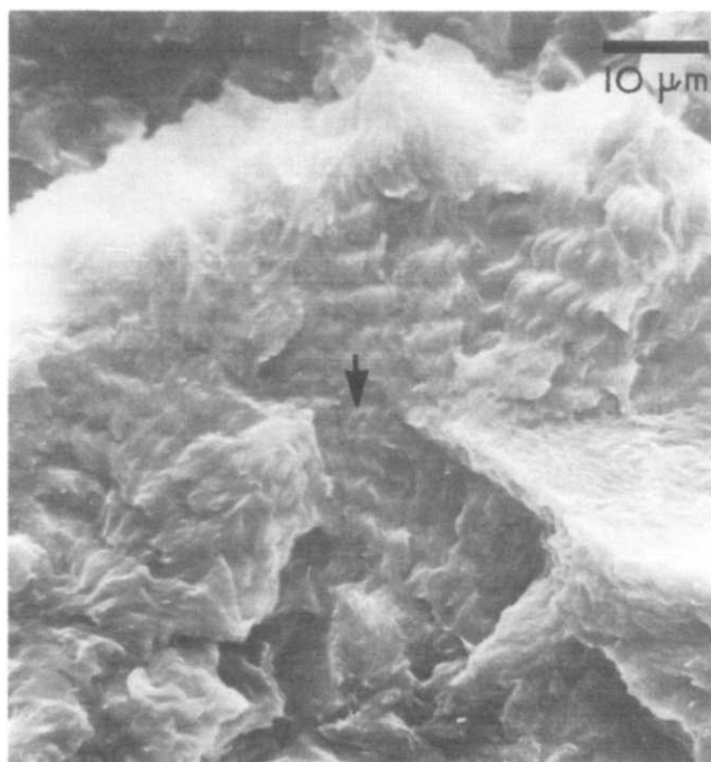
Figure 8 Interspherulitic crack propagation; also showing a smooth crack propagation across a matching interface (shown by arrow). Scale, 10 μm
